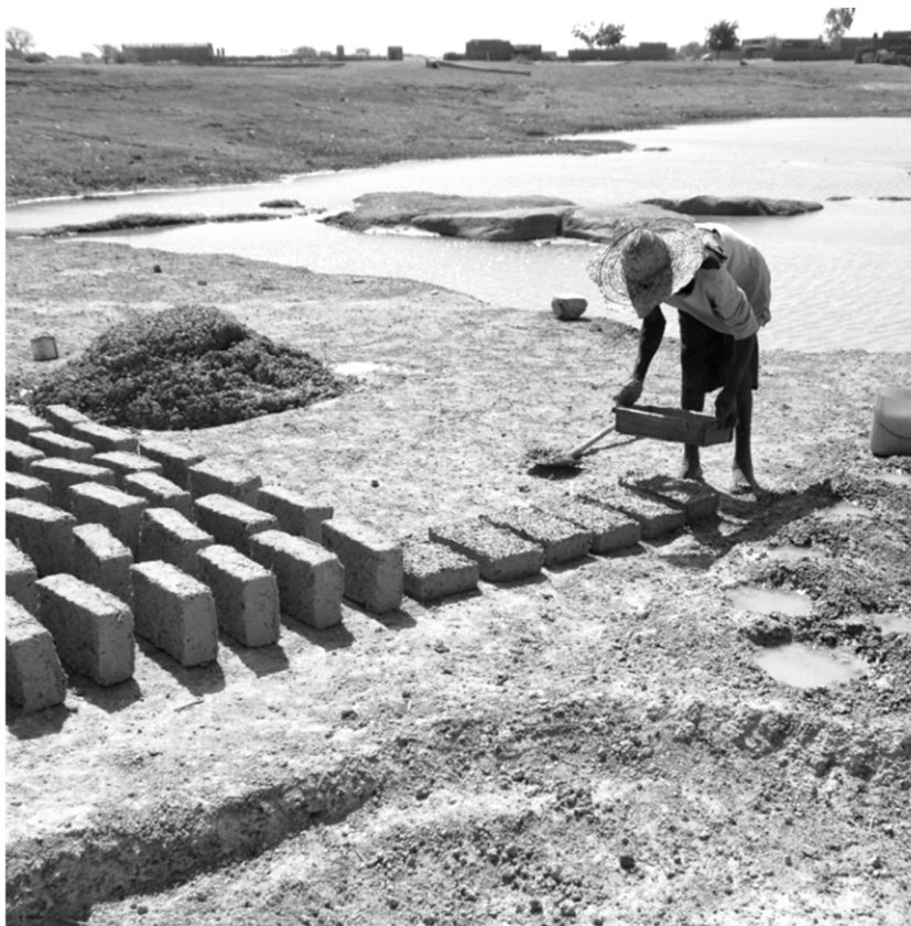
Figure 4. Adobe brick making with a timber-framed mould in Yemen; [2].
